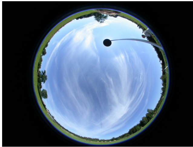
Figure 2. An hemispherical image taken with leveled camera from tripod. The field of view extends below horizon. The direct radiation from the Sun is screened to avoid artifacts due to significant scattering in the optical system.
